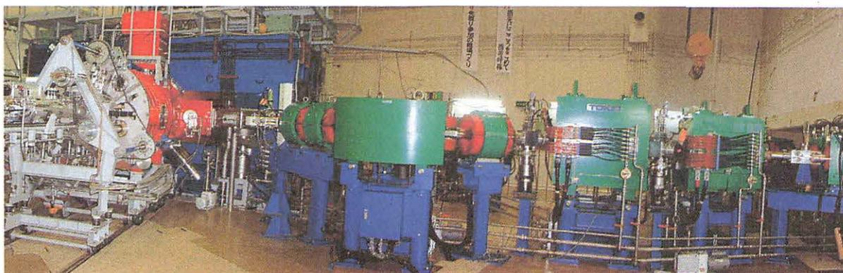
Photograph pictures the new AVF cyclotron and beam extraction ports in the cyclotron vault.
