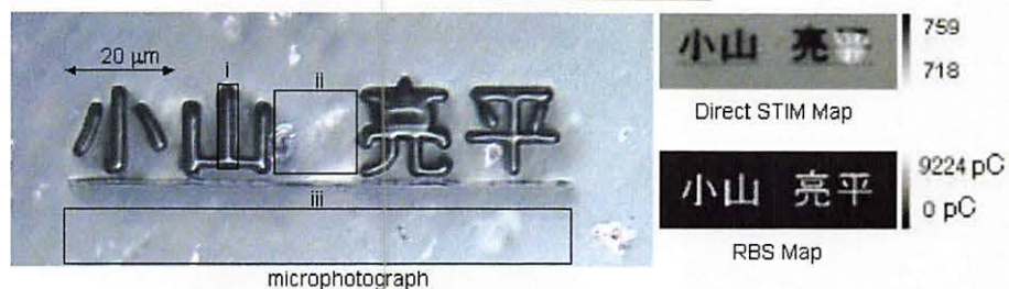
Figure 8. Microphotograph, RBS Map, and Direct STIM Images of a Mylar film after Irradiation with a Scanning Pattern of Chinese Characters: 小山 亮平.
