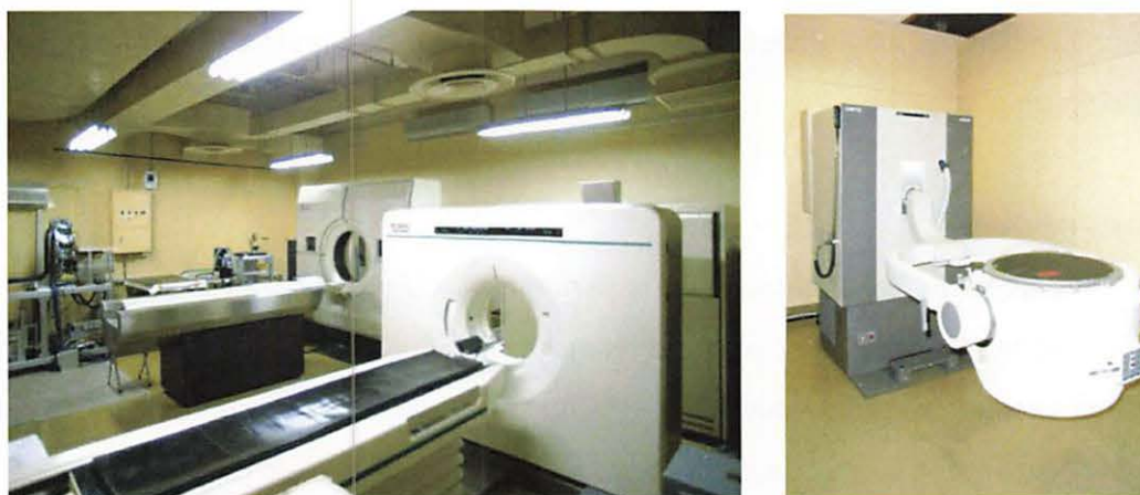
Figure 1. Nuclear medicine systems for animals. Left figure shows PET systems. From the left, ultra-high resolution semiconductors PET system, PT-931-04 PET system, HEADTOME-IV PET system. Right figure shows ZLC-7500 gamma camera.
