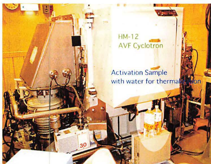
Figure 3. Irradiation by thermal neutrons from K=12 MeV -AVF cyclotron. Samples are mounted between two bottles filled with water located at the right under the RI-production target.
