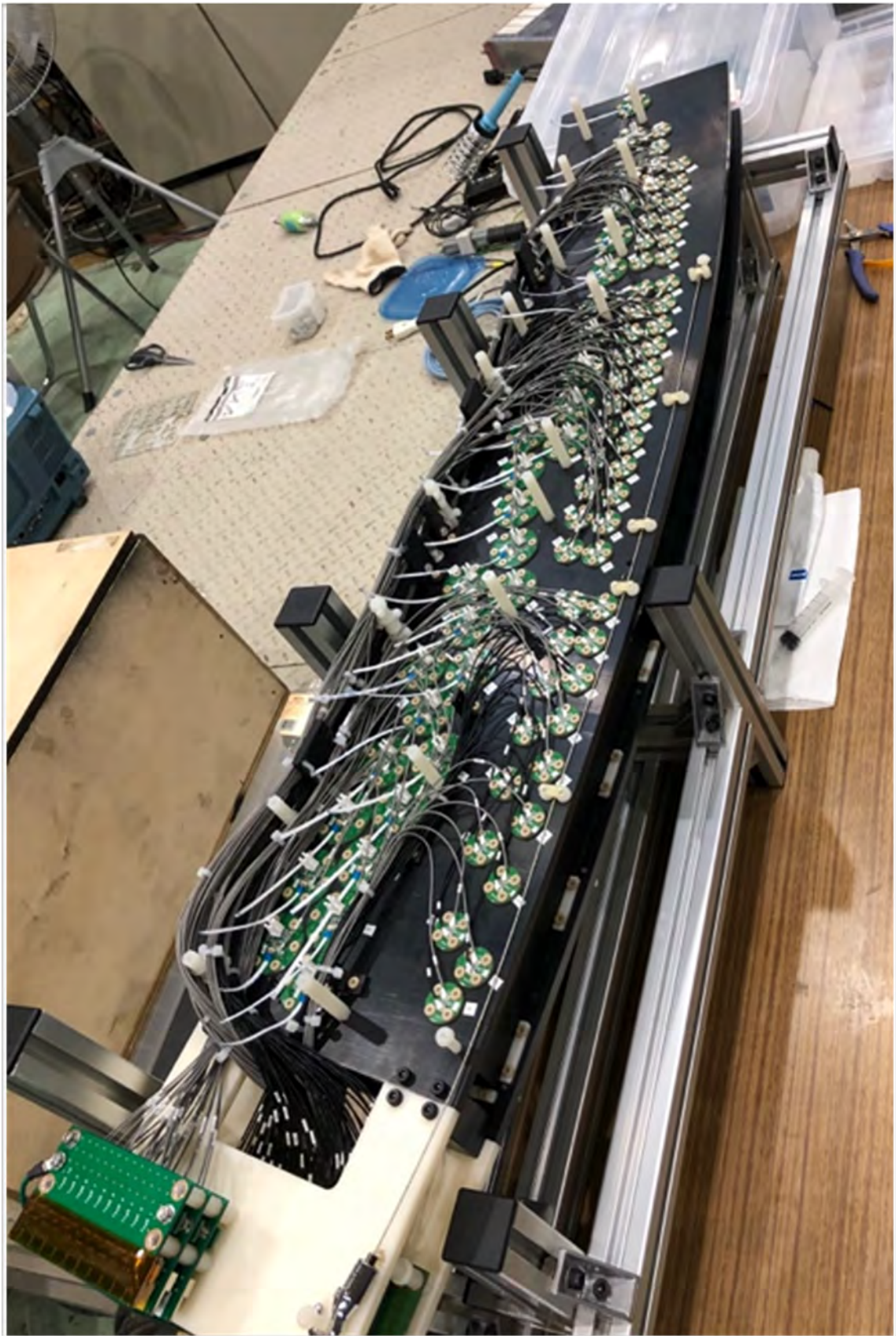
Fig.7. A picture of the tagger assembled. The tagger is placed in a frame made of aluminum to prevent it from tipping over. The upper side in photo related to a part which goes into the back of the dipole magnet. The other edge will locate the entrance side of the magnet. Note that the power supply PCB is not mounted in the picture.
