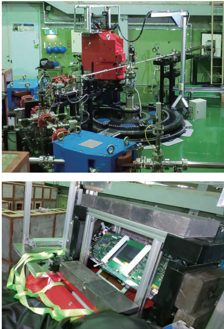
Fig.1. Picture of the ULQ2 beam line and spectrometer (top) and focal plane detector and lead shield at the top of the spectrometer (bottom).
